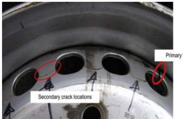
Fig. 4. Failure during RFT
